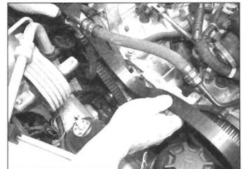
7.15b Removing the primary timing belt
