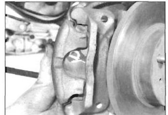
12.7 Remove caliper assembly and secure it safely to one side
