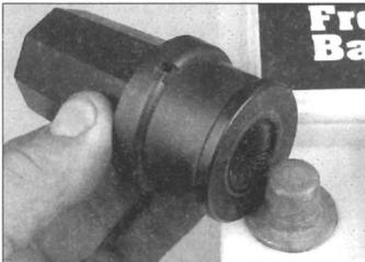
**3** If corrosion (white, fluffy deposits) is evident, remove the cables from the battery terminals, clean them with a small wire brush, then refit them. Automotive stores sell a tool for cleaning the battery post . . .
