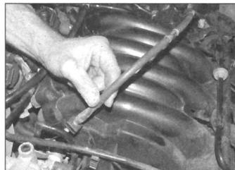
**10.5 Disconnect the accelerator cable from the throttle linkage**
