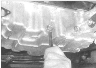
3.5 Slackening the engine oil drain plug
