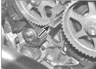
7.6b Sprocket locking tool in position
