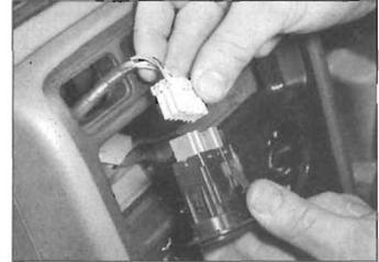
29.13d . . . and disconnect the wiring
