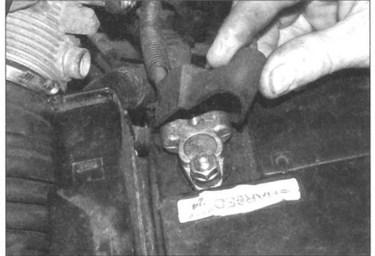
**2** Check the tightness of the battery cable clamps to ensure good electrical connections. You should not be able to move them. Also check each cable for cracks and frayed conductors.
