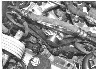
7.15a Note the routing of the belt before removal
