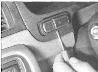
4.7c Using a screwdriver, prise out the foglight switch ...
