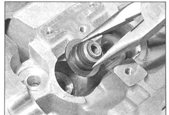
**7.3b** Extracting the spring lower seat/stem seal
