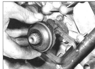
6.2 Removing the clutch release bearing – R65-type transmission
