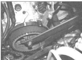
7.31 ... but the rear sprocket must be turned using a home-made forked tool
