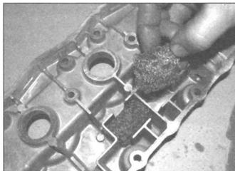
4.8 Ensure that the oil separator meshes are clean
