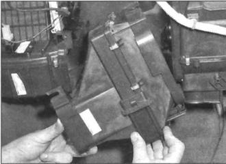
9.8 . . . and withdraw the air duct
