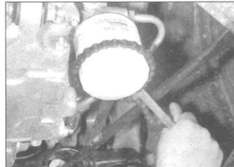
3.10 Loosening the oil filter using an oil filter removal tool
