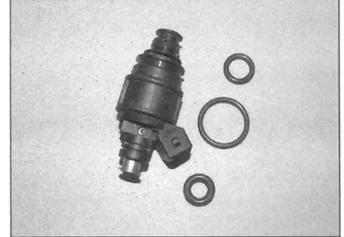
11.10 Each injector should have three new O-rings
