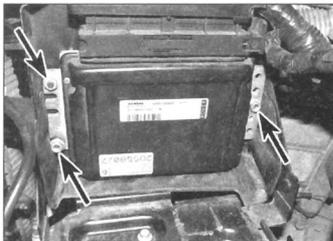
**11.66 Undo the three mounting nuts – arrowed**
