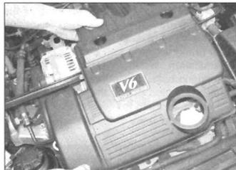
4.1b . . . and lift off the engine top cover
