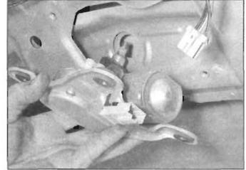
22.6b . . . and remove the tailgate wiper motor
