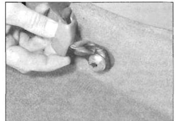
27.6 Front seat belt lower mounting bolt on the inner sill panel
