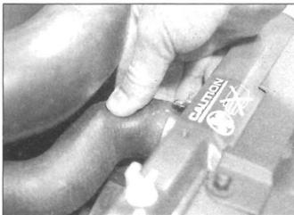
10.1 Checking the condition of a coolant hose
