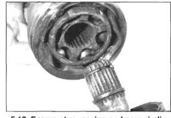
5.12 Ensure stopper ring and new circlip are correctly located before fitting outer CV joint
