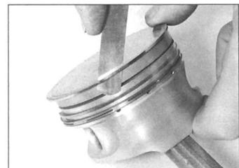
14.2 Using a feeler blade to aid removal of the piston rings
