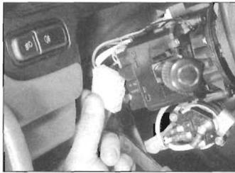
4.3 Disconnecting the wiring multiplugs from the wiper/lighting switches
