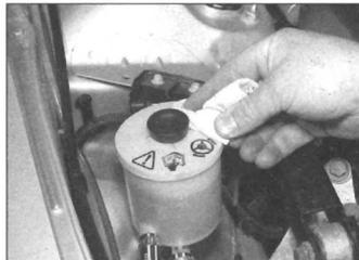
**2** If topping-up is necessary, first wipe the area around the filler cap with a clean rag before removing the cap.
