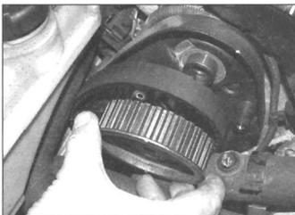
7.42b . . . then remove the inlet sprocket . . .
