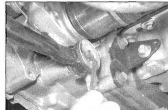
3.18a Unscrew the bolt securing the gearchange steady rod to the transmission . . .
