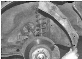
25.2b Removing a rear wheel arch liner
