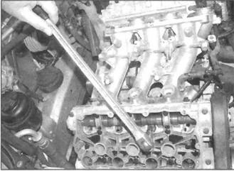
11.17a Loosen the head bolts in sequence
