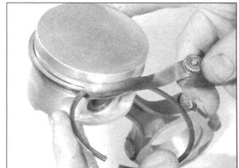
18.9 Measuring piston ring-to-groove clearance
