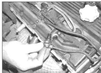
11.57 Remove the camshaft position (CMP) sensor
