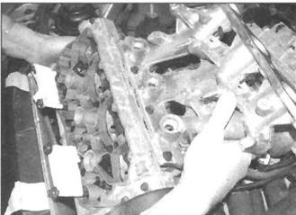
11.20 Lifting off the head – note front bolts wrapped up with tape
