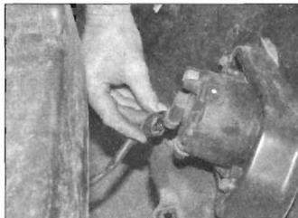
6.6b Disconnecting the wiring from the foglights when removing the front bumper
