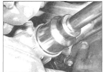
4.6 Fitting a driveshaft oil seal using a socket – R65-type transmission
