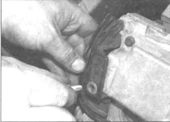
4.4 Unbolt and remove the HT lead guide clip
