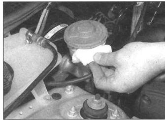
**2** If topping-up is necessary, wipe the area around the filler cap with a clean rag before removing the cap. Before topping-up, it is a good idea to inspect the reservoir. The system should be drained and refilled (see Chapter 9) if deposits, dirt particles or contamination are seen in the fluid. Pour fluid carefully into the reservoir to avoid spilling it on surrounding painted surfaces.
