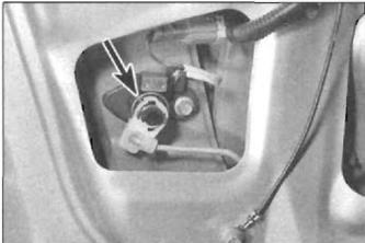
19.12 Tailgate lock cylinder accessible through the aperture in the tailgate inner panel
