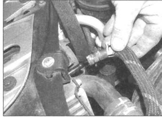
11.8a Disconnect the expansion tank hose from the radiator ...
