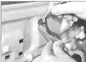
14.15a Releasing the wiring from the clip
