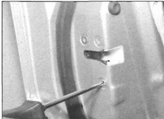
13.25 Unscrewing the front door lock mounting screws
