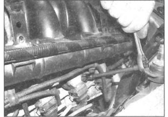
12.12 Unscrew the bolts from the two manifold rear support brackets
