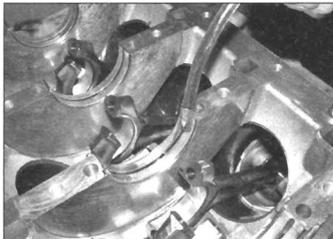
**19.23** Lubricate the bearing shells in the cylinder block with clean engine oil
