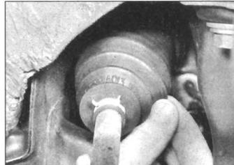
**17.2 Checking the condition of a steering gear rubber gaiter**
