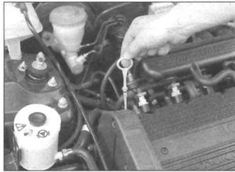
**1** The dipstick is located at the right-hand end of the engine, at the rear of the engine on 4-cylinder petrol models, and at the front of the engine on 6-cylinder petrol and diesel models (see *Underbonnet check points*). Withdraw the dipstick.
