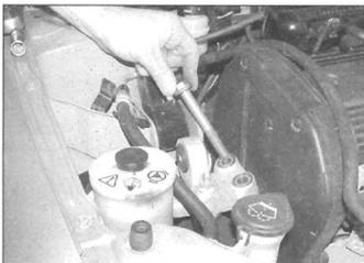
7.9b ... remove the mounting bracket bolts ...
