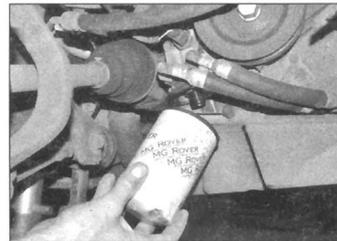
**3.8b** Oil filter location – 6-cylinder engines
