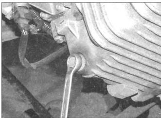
3.5a Slackening the engine oil drain plug – 4-cylinder engines
