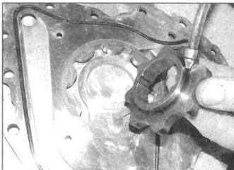
15.11 Lubricate the pump rotors before fitting them
