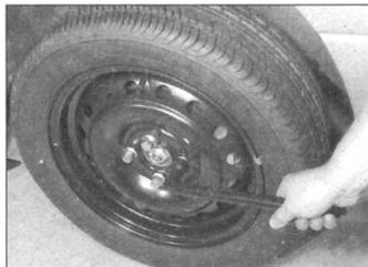
**8** Lower the car to the ground and tighten the wheel nuts in a diagonal sequence. Where applicable refit the wheel trim.
