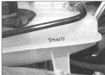
**1** The coolant level varies with the temperature of the engine. When the engine is cold, the coolant level should be on the MAX marking on the side of the reservoir. When the engine is hot, the level may rise slightly.
