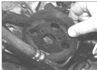
6.9 Removing the power steering pump pulley
