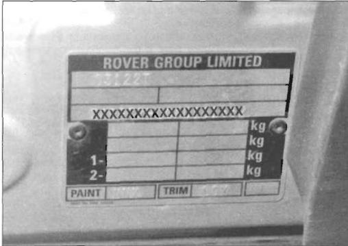
Vehicle identification plate on passenger door pillar
