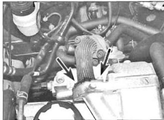
**4.2** Remove the EGR cooler pipe bolts (arrowed)
