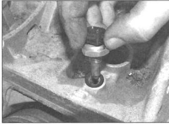
11.26b . . . then unscrew and remove the coolant temperature sensor
