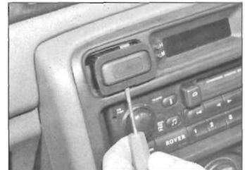
4.7a Using a screwdriver, prise out the hazard switch ...
