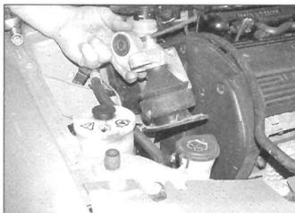
7.9c ... and withdraw the mounting assembly
