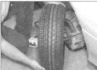
**7** Fit the spare wheel into position and tighten the nuts moderately with the wheelbrace.
