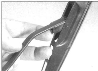
**2** To remove a wiper blade, pull the arm fully away from the glass until it locks. Swivel the blade through 90°, press the locking tab with a finger nail and slide the blade out of the arm's hooked end. On refitting, ensure that the blade locks securely into the arm.
