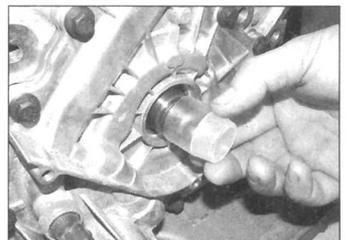
14.12 Fit the oil seal fitting sleeve in place
