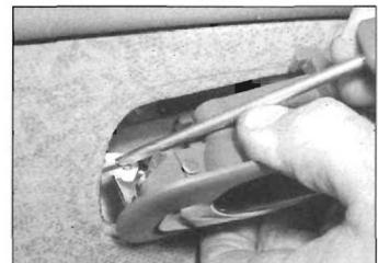
12.13 Slide the interior door handle forwards and disconnect the operating rod
