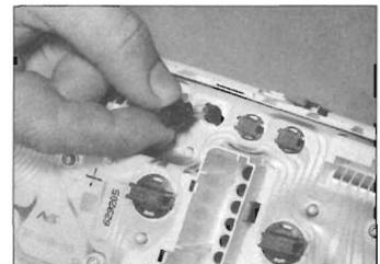
6.11c Removing a warning lamp bulbholder ...
