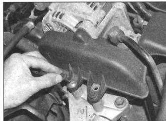
**6.26 Undo the two cover retaining bolts**
