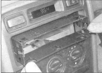
29.13b . . . and remove the radio mounting box
