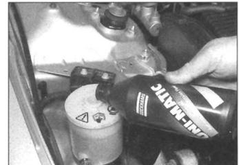
**3** When adding fluid, pour it carefully into the reservoir to avoid spillage – be sure to use only the specified fluid. After filling the reservoir to the correct level, make sure that the cap is refitted securely to avoid leaks and the entry of foreign matter into the reservoir.
