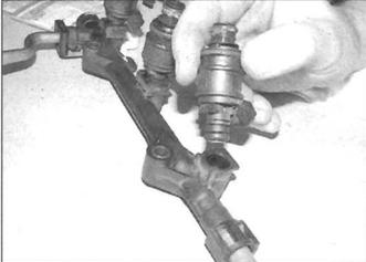
11.9b . . . then ease each injector out of the fuel rail
