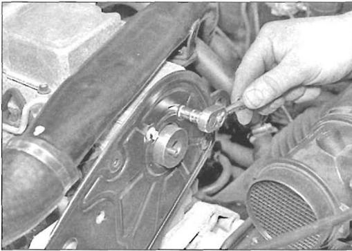
13.4a Unscrew the securing bolts ...
