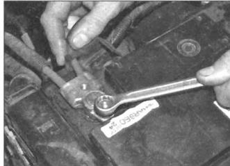
**B** Check the security and condition of the battery connections.
