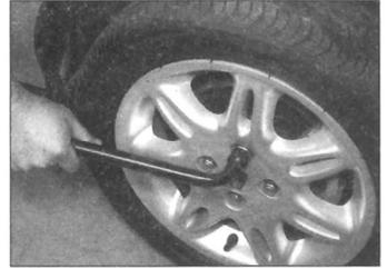
**3** Slacken each of the wheel nuts by half a turn, using the special adaptor on the locking wheel nut.
