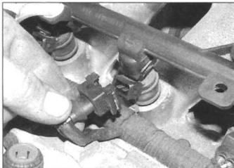
11.7a Disconnect the injector wiring plugs
