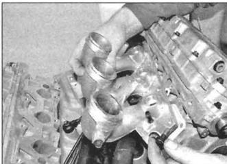
**12.31b** . . . then refit the rear manifold, and tighten the bolts
