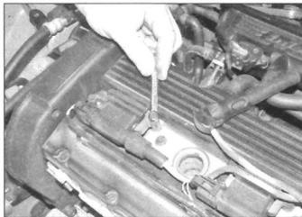
3.4 Remove the two coil bolts . . .
