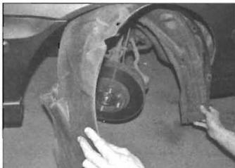
25.2a Removing a front wheel arch liner
