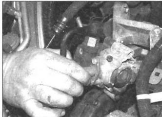
7.6b . . . and lift the pump off the engine front plate
