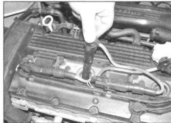
3.3 Pull the HT lead connector from the spark plug
