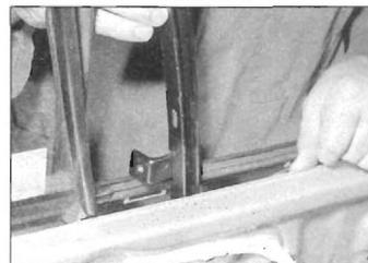
14.13c ... then twist the channel through 90° and lift from the door
