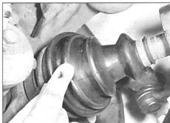
**16.1 Inspecting a driveshaft joint rubber gaiter**
