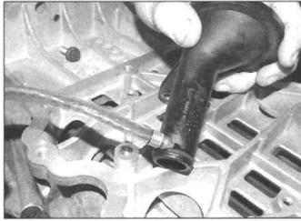
12.12b . . . then oil and refit the oil pump pick-up
