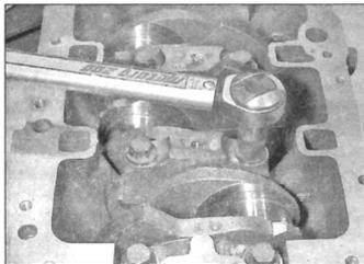
17.9 Tighten the main bearing cap bolts to the specified torque
