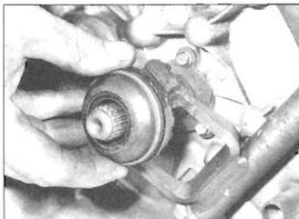
4.11 Remove the release bearing
