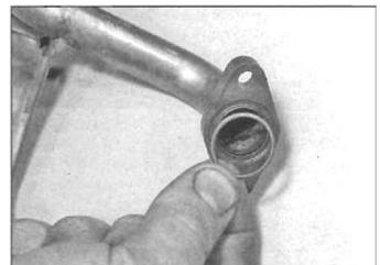
15.12 Refit the oil pump pick-up/strainer pipe using a new O-ring
