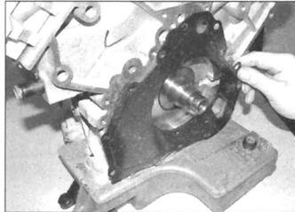
14.9 Fit the new oil pump gasket
