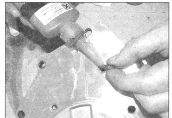
15.12 Thread-lock the oil pump cover screws
