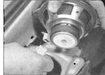
24.6b ... and disconnect the wiring from the rear speaker
