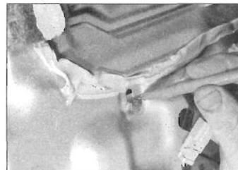
14.15b Marking the position of the regulator mounting bolts
