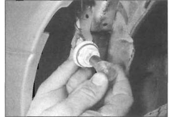
5.18 ... and remove the front direction indicator bulb
