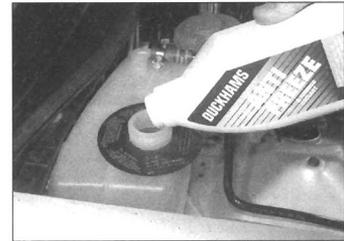
**3** Add coolant (a mixture of water and antifreeze) through the expansion tank filler neck, until the coolant is up to the MAX level. Refit the cap; turning it clockwise as far as it will go until it is secure.
