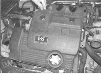
4.1 Removing the engine acoustic cover
