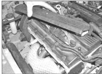
26.6 Remove the coil/plug cover
