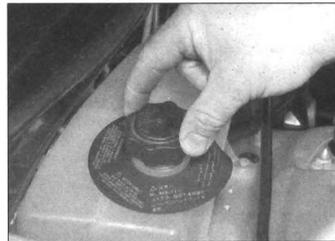
**2** If topping-up is necessary, wait until the engine is cold, then cover the expansion tank cap with a rag and unscrew the filler cap anti-clockwise. Wait until the hissing ceases, indicating that all pressure is released, then unscrew and remove the filler cap.
