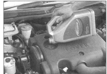
**4** Oil is added through the filler cap. Rotate the cap through a quarter-turn anti-clockwise and withdraw it. Top-up the level. A funnel may help to reduce spillage. Add the oil slowly, checking the level on the dipstick often. Do not overfill.
