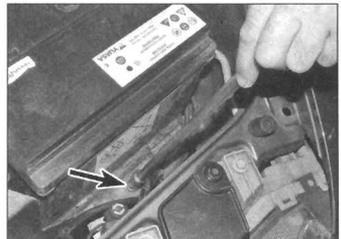
3.4a Unscrew the bolt (arrowed) to remove the retaining clamp . . .
