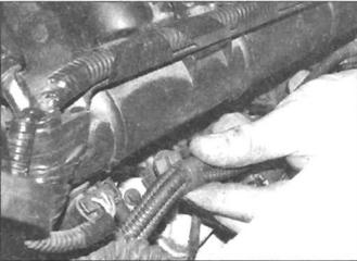
12.13 Unclip the rear ignition coil wiring harness from the manifold
