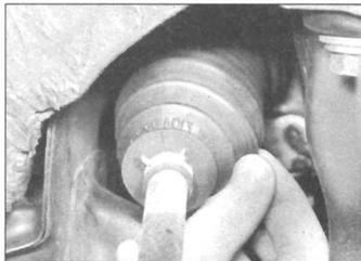
17.2 Checking the condition of a steering gear rubber gaiter
