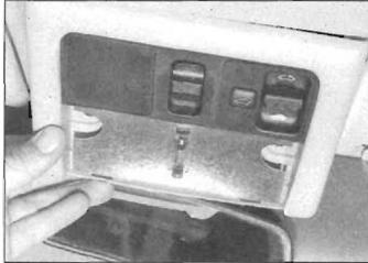
4.42b . . . and withdraw the interior light assembly
