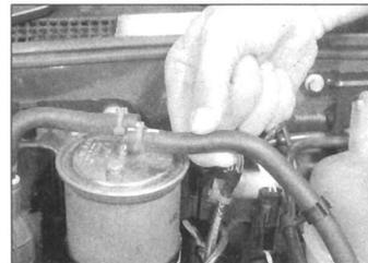
10.5 Check for fuel leaks at the fuel filter unions
