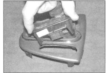
4.2 Squeeze the tabs under the panel and remove the selector indicator
