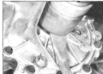
3.9 Carefully lever driveshaft inner CV joint out of housing
