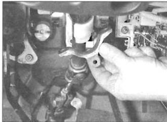
14.8b . . . and remove the mounting clamp
