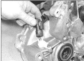
6.4 Removing the vehicle speed sensor
