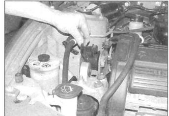
7.9a Tilt the steady bar upward ...
