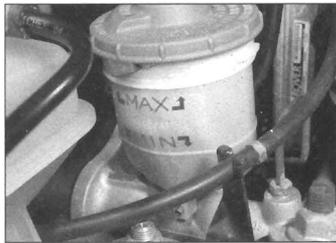
**1** The brake master cylinder and fluid reservoir is located at the rear right-hand end of the engine compartment. The MAX and MIN level marks are indicated on the side of the reservoir and the fluid level should be maintained between these marks at all times.
