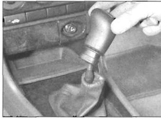
29.11 Removing the gear knob
