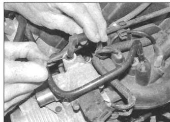
**10.4a Release the locking collar to disconnect the vacuum pipe . . .**
