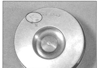
12.21c . . . should be positioned to the left of the arrow on the piston crown when the piston is viewed from the flywheel end
