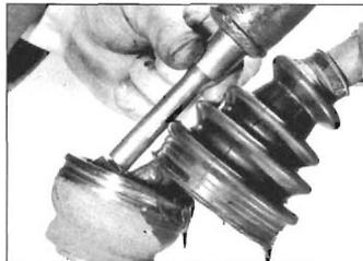
5.4 Driving outer CV joint off driveshaft end
