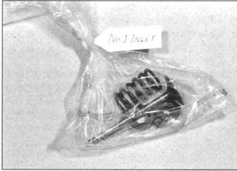
**7.5 Use a labelled plastic bag to keep together and identify the valve components**
