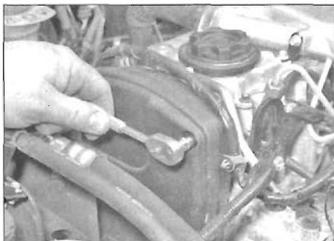
**6.1a** Unscrew the securing bolts . . .
