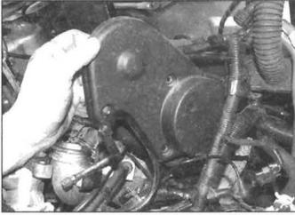
6.24 Removing the secondary belt rear bank cover
