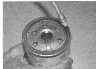
**3.12** Apply clean oil to the seal on the oil filter
