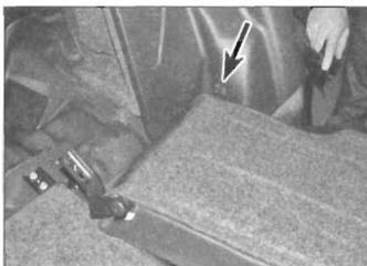
26.15b . . . disengaging it from the outer hinge pin – arrowed
