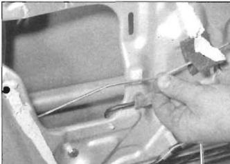
13.22 Releasing the front door lock operating rod from the guide
