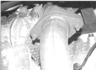
12.5b Exhaust front manifold-to-downpipe nuts
