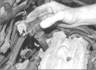
4.5b . . . and withdraw the coil
