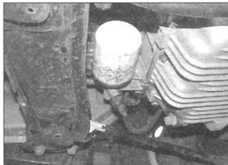
**3.8a** Oil filter location – 4-cylinder engines
