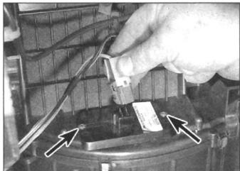
9.28a Disconnect the wiring connector, undo the two screws (arrowed) ...
