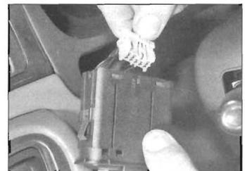
4.7d ... then disconnect the wiring multiplug
