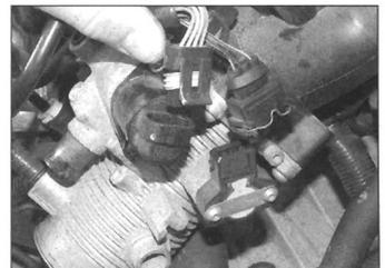
**10.8 Disconnect the throttle sensor and air valve wiring plugs**
