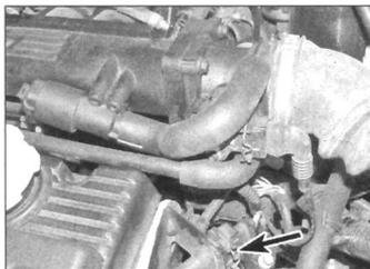
11.48 Disconnect the wiring connector – arrowed
