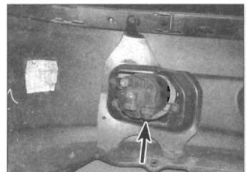
7.25 Insert screwdriver in position shown (arrowed) to adjust foglamp
