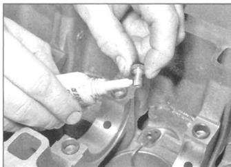
**11.11 Apply thread-locking fluid to the oil spray jet securing bolts**
