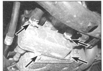
17.5 Oil cooler coolant hoses and mounting bolts
