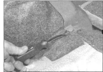
28.1b Removing a stud fixing
