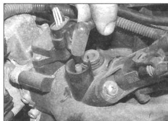
**12.5b ... and pull off the vacuum pipe from the throttle body ...**
