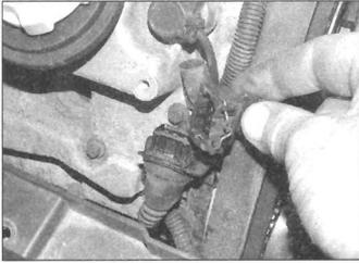
11.47a Disconnect the wiring plug connector . . .
