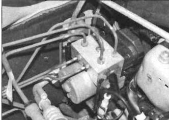
25.7 Anti-lock braking System (ABS) modulator
