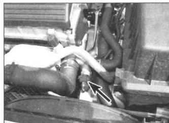
11.23 Engine coolant temperature (ECT) sensor location
