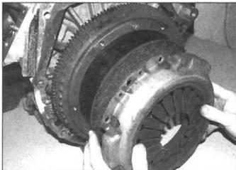
5.5 Withdraw the pressure plate and friction disc – 6-cylinder engine shown
