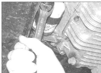
**3.10** Slackening the filter using an oil filter removal tool
