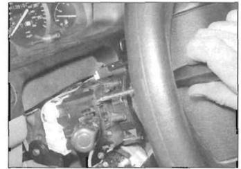
4.4a Undo the switch mounting screws ...
