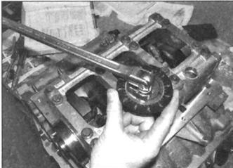
19.29b . . . using an angle gauge . . .
