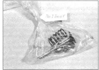
6.5 Place each valve assembly in a labelled polythene bag
