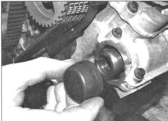
7.21 Remove the exhaust camshaft end caps
