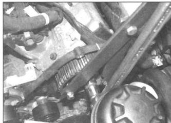
8.2 Use a home-made tool to hold the sprocket
