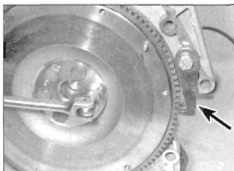
**19.3** Unscrewing a flywheel bolt – note bolt (arrowed) to prevent flywheel from turning
