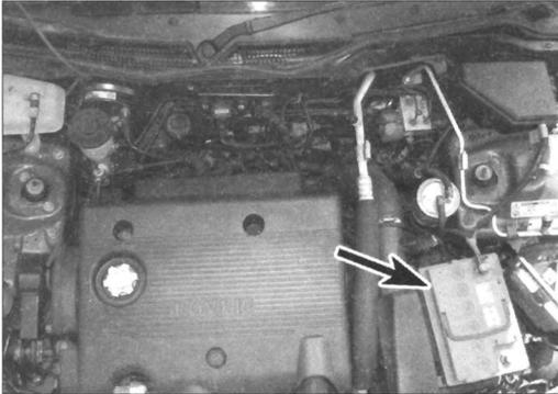
**1** The battery is located on the left-hand side front of the engine compartment. The exterior of the battery should be inspected periodically for damage such as a cracked case or cover.
