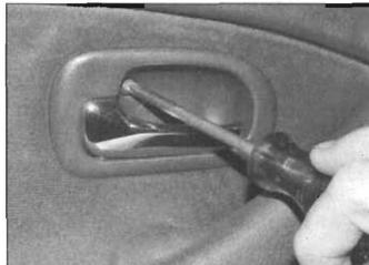
12.3 Undo the screw securing the interior door handle to the door inner panel . . .
