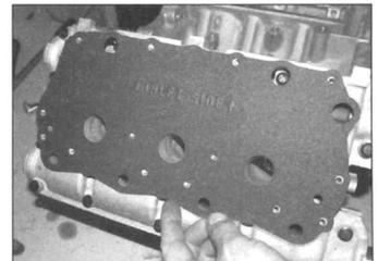
4.9 Observe the direction-of-fitting marks on the new gasket
