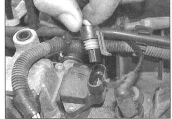
11.51 Disconnecting the MAP sensor wiring plug
