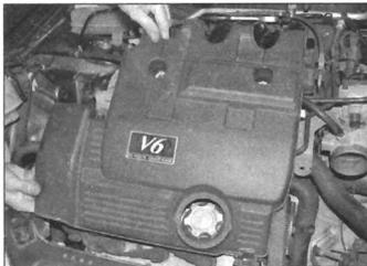
26.3 Remove the engine cover – 6-cylinder engines
