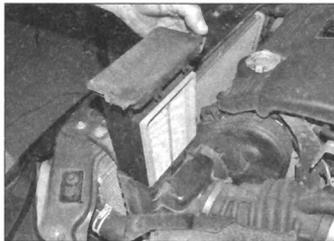
25.6a Slide the air filter cartridge from the housing ...
