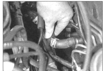
**9.2 Disconnecting the supply and return hoses on engine compartment bulkhead**
