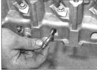
3.5 Remove the glow plugs from the cylinder head
