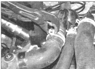
**4.11** Remove the hoses from the thermostat housing
