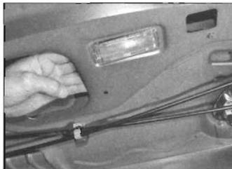
6.6 Releasing the boot light retaining clip
