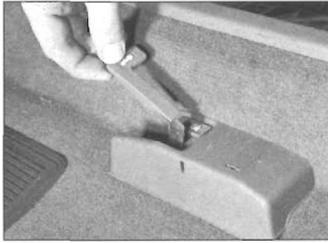
17.3 Pull off the control knobs ...
