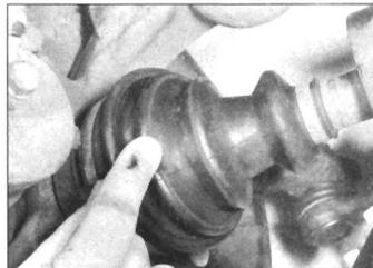
**16.1 Inspecting a driveshaft joint rubber gaiter**
