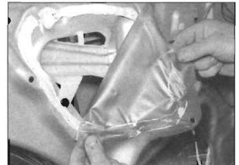
**12.18b** . . . and carefully peel away the membrane
