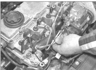
10.19 Removing the injector pipes
