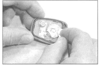
5.3 Fit the new battery, handling it with a piece of tissue paper to avoid touching the battery contact surfaces
