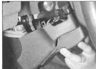
4.2b . . . and remove the steering column lower . . .
