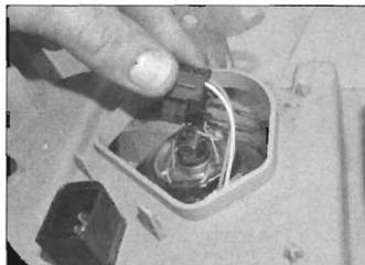
5.3a . . . unplug the wiring connector . . .
