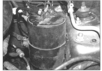
2.3b Charcoal canister – 6-cylinder engines
