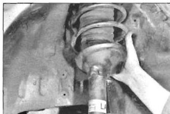
**4.7b . . . and withdraw the shock absorber/spring assembly from under the wheel arch**
