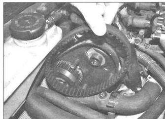
7.42c . . . and take the belt off the exhaust sprocket
