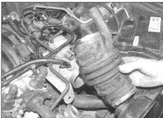
**10.3 Removing the inlet air duct**
