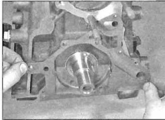
**16.15** Fit a new gasket to the cylinder block – viewed with engine removed
