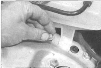
20.1 Temporarily unbolt the cooling system expansion tank and position it away from the bulkhead
