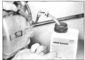
6.21 Using a one-way valve kit to bleed the braking system
