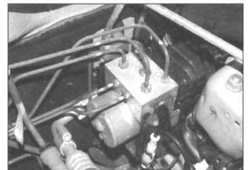
**10.15 Check the brake pipe unions on the ABS unit for leakage**
