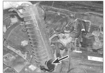
2.3a Disconnect air intake duct from lower part of housing – arrowed
