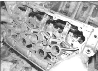
10.14 Refit the camshaft carrier onto the locating dowels
