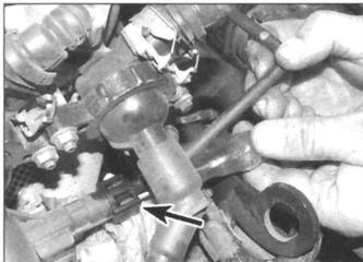
11.4 Use a small screwdriver to release the fuel rail rigid pipe
