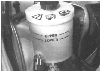
**1** The power steering fluid reservoir is located on the right-hand side of the engine compartment. UPPER and LOWER level marks are indicated on the side of the reservoir and the fluid level should be maintained between these marks at all times.
