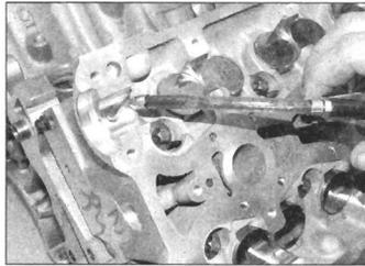
10.11 Oil the camshaft bearings in the cylinder head
