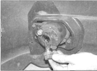
5.25 Twist the bulbholder to remove
