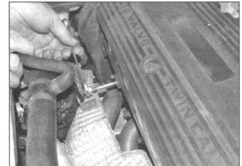
5.21 Using two nuts locked together to remove the bracket stud
