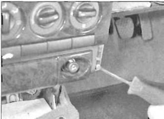
31.6a Undo the outer screws ...
