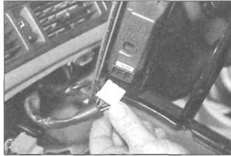
29.15 ... then withdraw the console and disconnect the wiring from the digital clock
