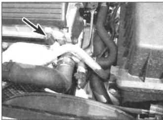
13.2c Low-pressure valve – 4-cylinder petrol models
