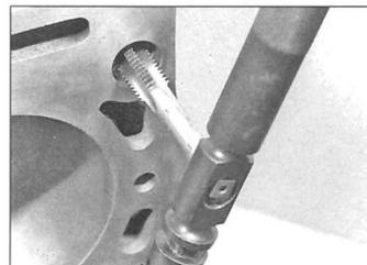
11.8 Clean out the threaded holes in the cylinder block using the correct-size tap
