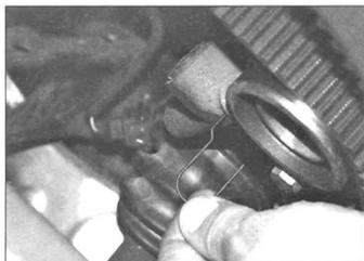
7.33b Removing the tensioner locking pin
