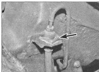
**7.5 Spring clip (arrowed) securing brake pipe connection**
