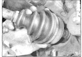
3.16 Engage the outer CV joint with swivel hub
