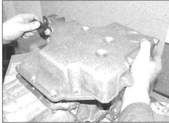
12.14 Offer the sump into place, and fit the bolts finger-tight
