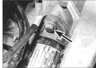
**8.8** Starter motor upper mounting bolt – arrowed
