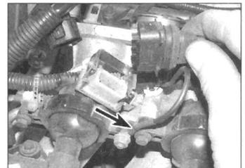
11.12a Disconnect the wiring plug – note earth lead (arrowed)
