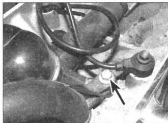
**4.13** Undo the bolt (arrowed) from the coolant elbow
