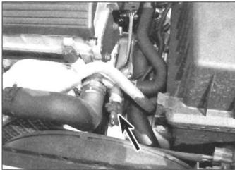
**8.3a Engine coolant temperature (ECT) sensor location – 4-cylinder petrol engines**
