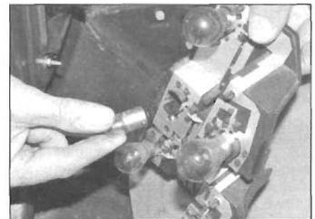
5.31 Removing a bulb from the rear light cluster
