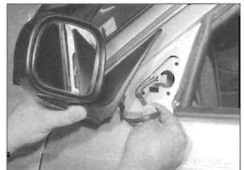
22.5b . . . and withdraw the mirror from the outside of the door
