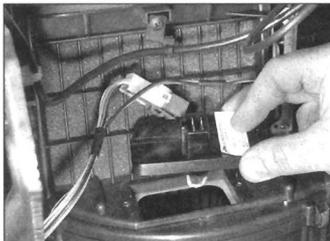
9.28b ... and withdraw the resistor
