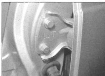
11.7 The door hinges are bolted to the A- and B-pillars
