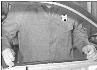
14.4 Removing the window glass from the front door
