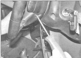
13.4 Undo the two airbag retaining screws
