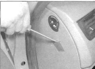
**31.19** Carefully prise out the side covers for access to the facia side mounting bolts
