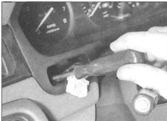
11.4a Undo the instrument panel surround lower mounting screws . . .
